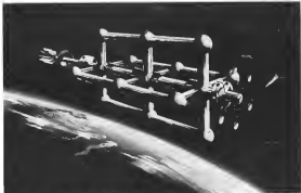
ADVANCED MODULAR design for earth-orbiting space station proposed by Lockheed Martin and Space Division scientists, will be assembled in space and orbit the earth at 310 mi. Station would consist of prefabricated parts connected into orbit.
